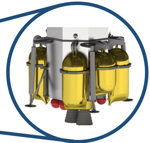
Drop Tanks (9.7 tons) Repurposed, then matured to full reusability
