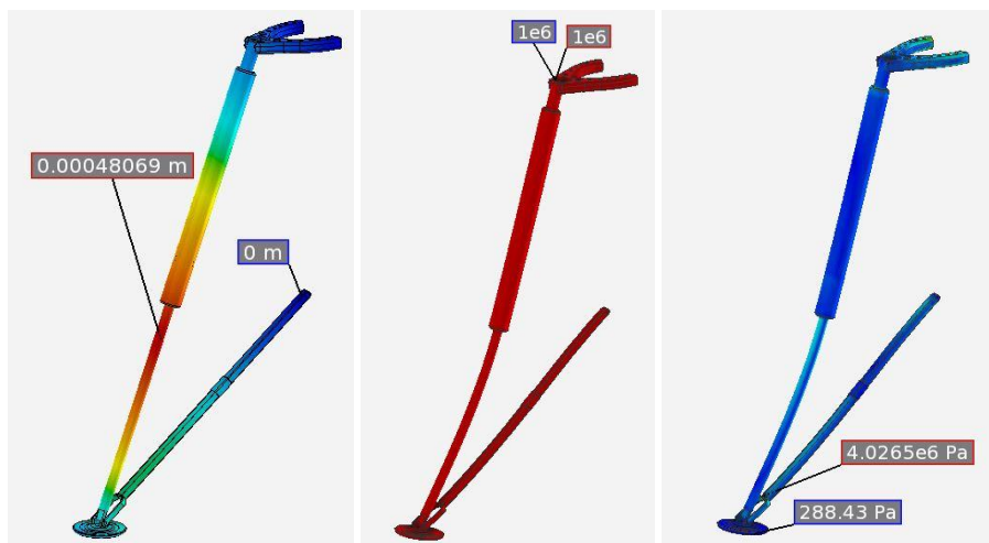
Figure 4: The structural simulation results for the landing legs.
